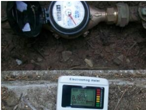
Smart water meter shows two spikes at peak of 2.4 milliwatts per meter squared (mwm 2 ). Close-up below.
